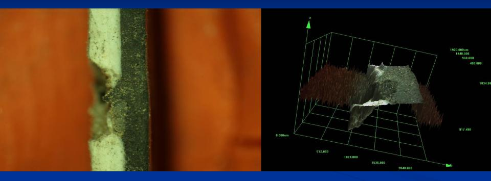
A change in the color of the waterproofing surface as a signal of degradation, in this case for single ply waterproofing.
