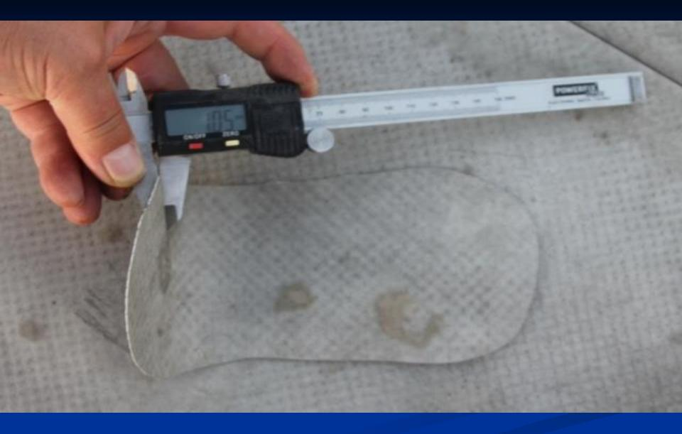
Asphalts and foam thermal insulation are not compatible with single ply waterproofing
